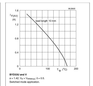
Fig.3 Maximum permissible average forward current as a function of tie-point temperature (including losses due to reverse leakage).
