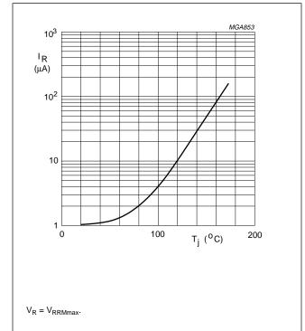
Fig.16 Reverse current as a function of junction temperature; maximum values.
