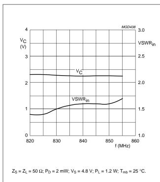
Fig.6 Control voltage and input VSWR as functions of frequency; BGY119A; typical values.
