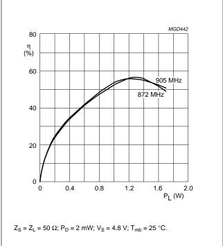
Fig.10 Efficiency as a function of load power; BGY119B; typical values.
