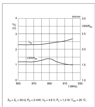
Fig.13 Control voltage and input VSWR as functions of frequency; BGY119B; typical values.
