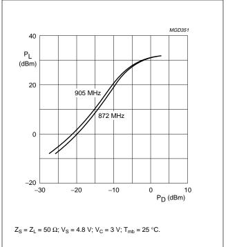
Fig.14 Load power as a function of drive power; BGY119B; typical values.
