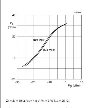
Fig.7 Load power as a function of drive power; BGY119A; typical values.
