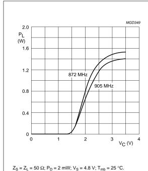
Fig.9 Load power as a function of control voltage; BGY119B; typical values.
