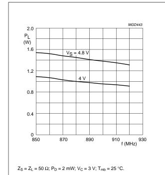
Fig.11 Load power as a function of frequency; BGY119B; typical values.
